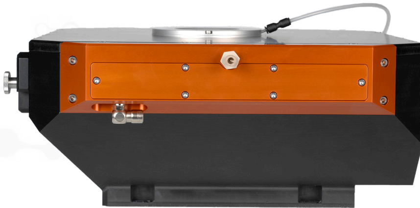
Figure 7. A side view of the TwoVol3 ablation cell showing the sample exit point.
