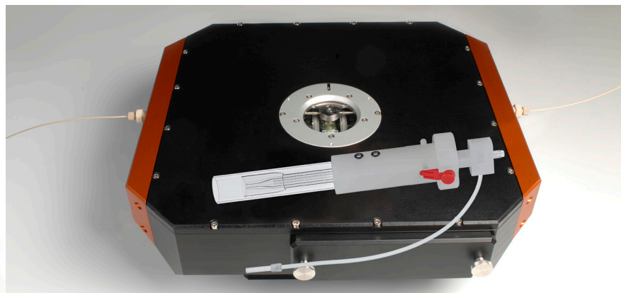
Figure 4. The TwoVol3 ablation cell in Imaging mode with the DCI.
